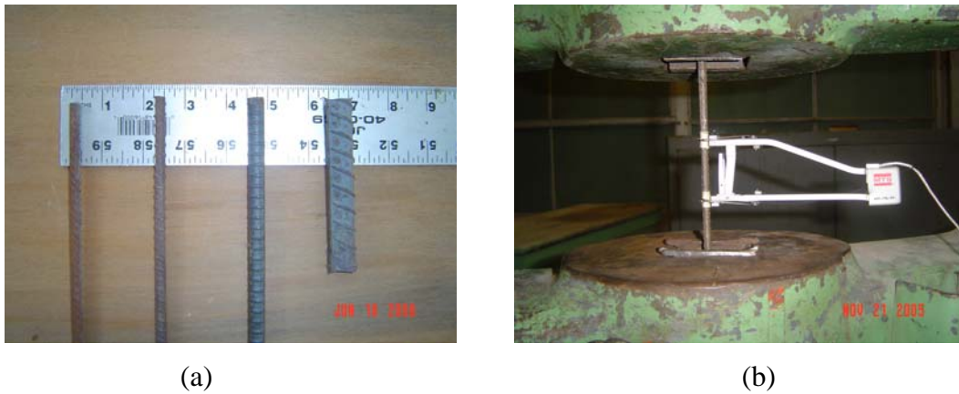
Fig. 3-8: (a) Tested rebar. (b) Tension test of a #3 rebar.
