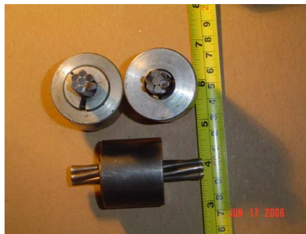
Fig. 3-9: Low relax. ½-in seven wire strand with wedges.
