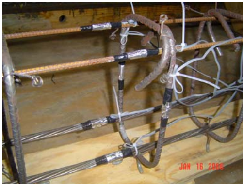
Fig. C-10: Installed strain gauges on longitudinal and transverse reinforcement.
