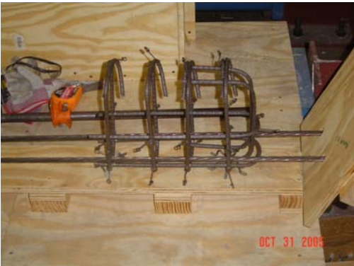
Fig. C-7: Reinforcement at beam ends.
