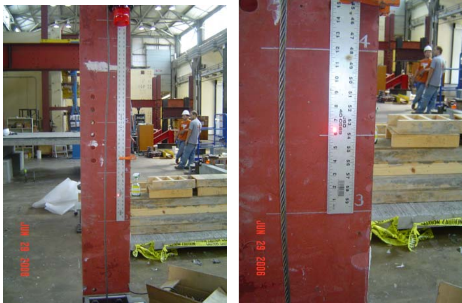
Fig. C-23: Scale used to measure the drop height of the pendulum mass.
