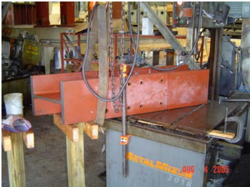
Fig. C-2: Cutting of W10×77.
