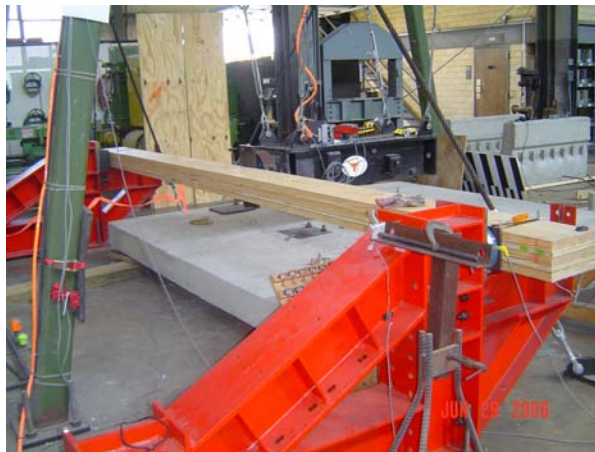
Fig. C-24: Test setup for laminated lumber beam.
