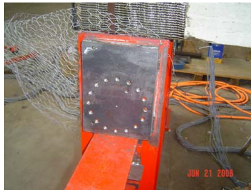
Fig. C-5: Base plate for load cell on A-frame.
