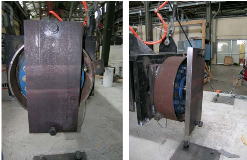
Fig. C-29: 200 kip load cell in front of pendulum mass.
