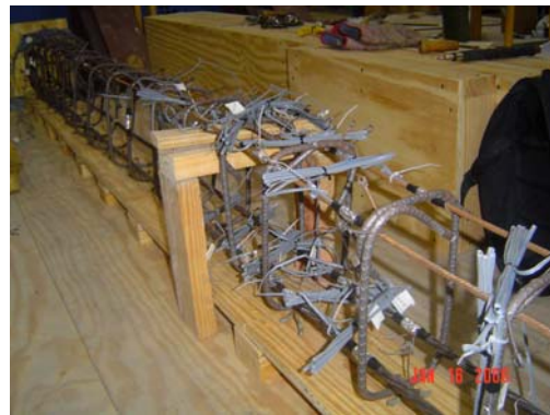
Fig. C-10: Installed strain gauges on longitudinal and transverse reinforcement.
