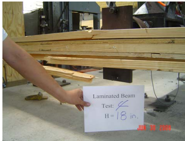
Fig. C-26: Failure of laminated lumber beam.
