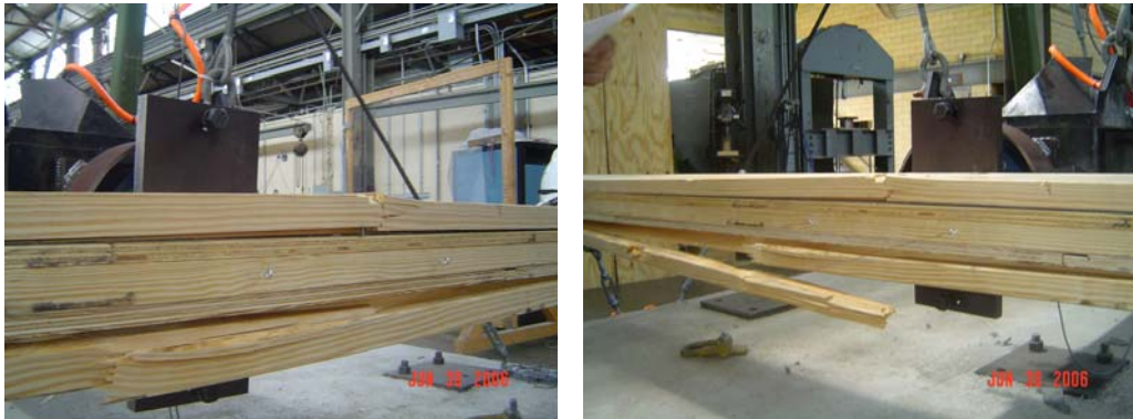
Fig. 5-24: Pictures of laminated lumber beam after final test.
