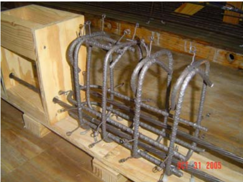
Fig. C-7: Reinforcement at beam ends.
