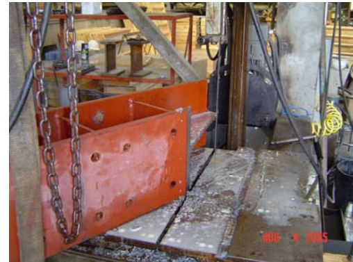
Fig. C-2: Cutting of W10×77.
