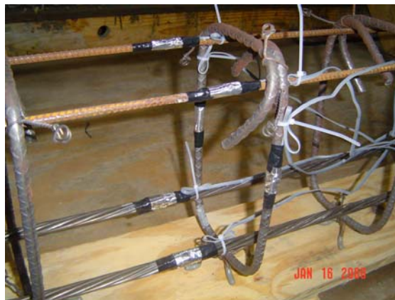
Fig. 4-18: Strain gauges on reinforcing steel and prestressing strand.
