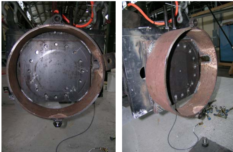
Fig. C-27: Protection ring for load cell in front of pendulum mass.
